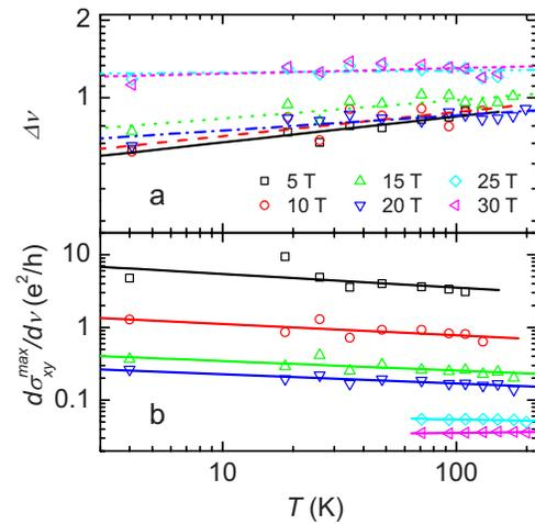
FIG. 4. (Color online) (a)  $\Delta\nu$ , distance between two extrema in the derivative  $d\sigma_{xx}/d\nu$  as a function of temperature for the zeroth Landau level. (b) The derivative  $(d\sigma_{xy}/d\nu)^{\max}$  as a function of temperature for the zeroth Landau level.
