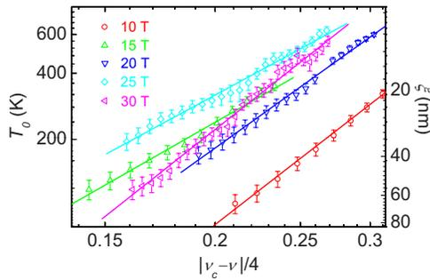
FIG. 3. (Color online) Scaling behavior in the tails of the first electron Landau level for various magnetic fields as a function of relative filling factor  $|\nu_c - \nu|/4$  with  $\nu = nh/eB$ . The factor 1/4 in the  $x$  axis accounts for the fourfold Landau level degeneracy. The localization length on the right axis was calculated by Eq. (4) with  $C=1$ .
