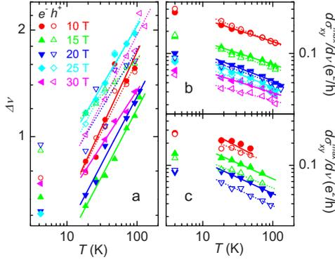
FIG. 2. (Color online) (a)  $\Delta\nu$ , distance between two extrema in the derivative  $d\sigma_{xx}/d\nu$  of the first electron Landau level (solid symbols) and the first hole (open symbols) Landau level for different magnetic fields. (b) The derivative  $(d\sigma_{xy}/d\nu)^{\max}$  as a function of temperature for the same levels. (c) The derivative  $(d\sigma_{xy}/d\nu)^{\max}$  as a function of temperature for the second electron and hole level.
